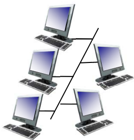
shared wire (e.g., cabled Ethernet)
