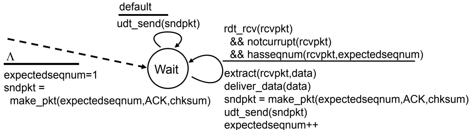
ACK-only: always send ACK for correctly-received pkt with highest *in-order* seq #
