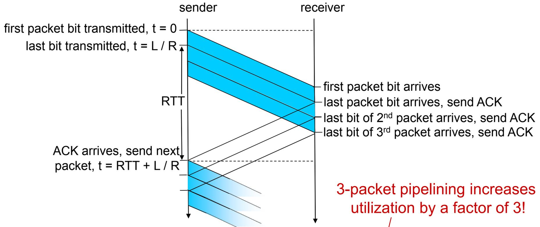
3-packet pipelining increases utilization by a factor of 3!
