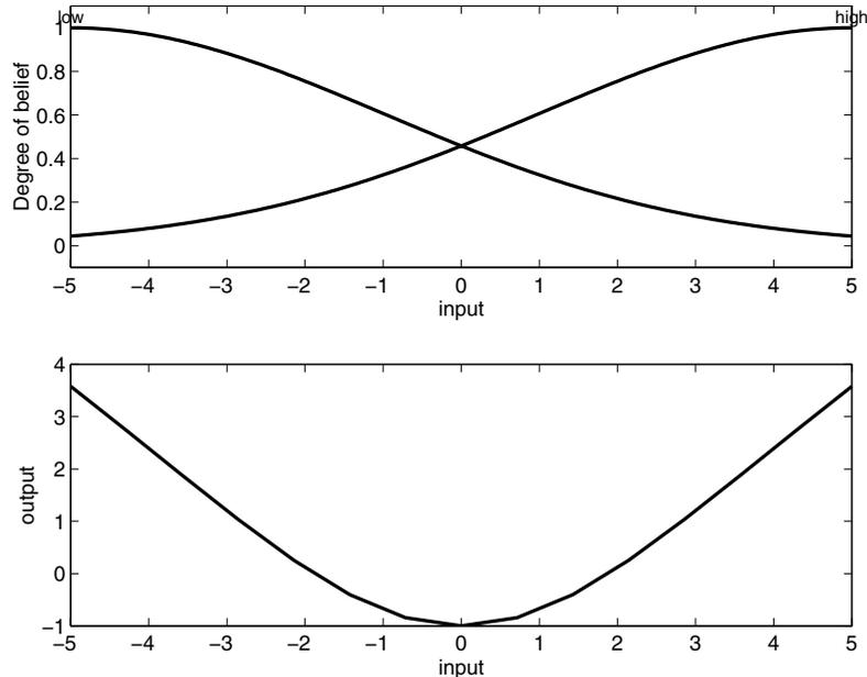
This is just one example of how a Sugeno-type system gives you the freedom to incorporate linear systems into your fuzzy systems. By extension, you could build a fuzzy system that switches between several optimal linear controllers as a highly nonlinear system moves around in its operating space.
