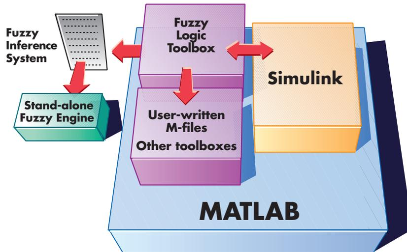
Because of the integrated nature of the MATLAB environment, you can create your own tools to customize the Fuzzy Logic Toolbox or harness it with another toolbox, such as the Control System Toolbox, Neural Network Toolbox, or Optimization Toolbox, to mention only a few of the possibilities.
