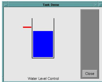
A controller for the water level in the tank needs to know the current water level and it needs to be able to set the valve. Our controller's input will be the water level error (desired water level minus actual water level) and its output will be the rate at which the valve is opening or closing. A first pass at writing a fuzzy controller for this system might be the following.
