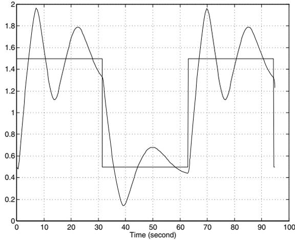
We need to add another input, the water level's rate of change, to slow down the valve movement when we get close to the right level.
