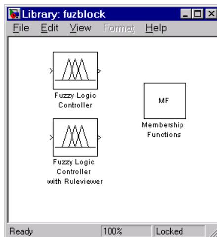
The Fuzzy Logic Toolbox library contains the Fuzzy Logic Controller and Fuzzy Logic Controller with Rule Viewer blocks. It also includes a Membership Functions sublibrary that contains Simulink blocks for the built-in membership functions.
