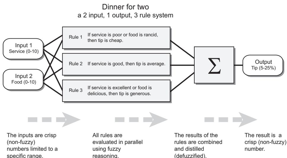
Information flows from left to right, from two inputs to a single output. The parallel nature of the rules is one of the more important aspects of fuzzy logic systems. Instead of sharp switching between modes based on breakpoints, we will glide smoothly from regions where the system's behavior is dominated by either one rule or another.
