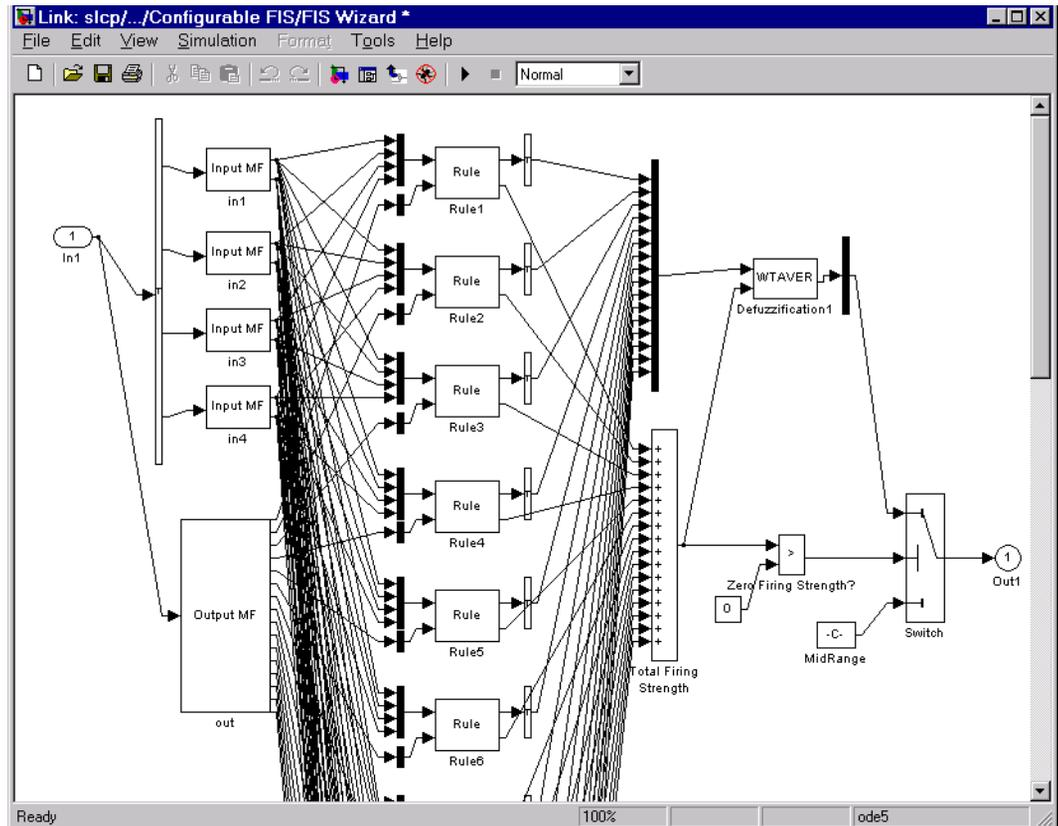
As the figure shows, the Fuzzy Logic Controller block uses built-in Simulink blocks to implement your FIS. Although the models can grow complex, this representation is better suited than the S-function `sffis` for efficient code generation.
