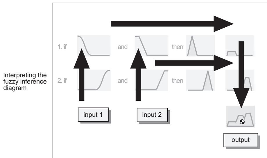
Notice how the flow proceeds up from the inputs in the lower left, then across each row, or rule, and then down the rule outputs to finish in the lower right. This is a very compact way of showing everything at once, from linguistic variable fuzzification all the way through defuzzification of the aggregate output.
